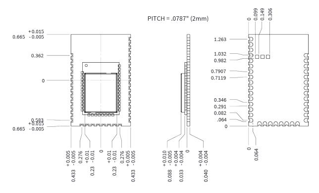
Mechanical drawings XBee 3 micro antennas
