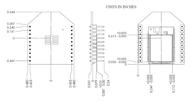
XBee 3 through-hole - U.FL antenna
