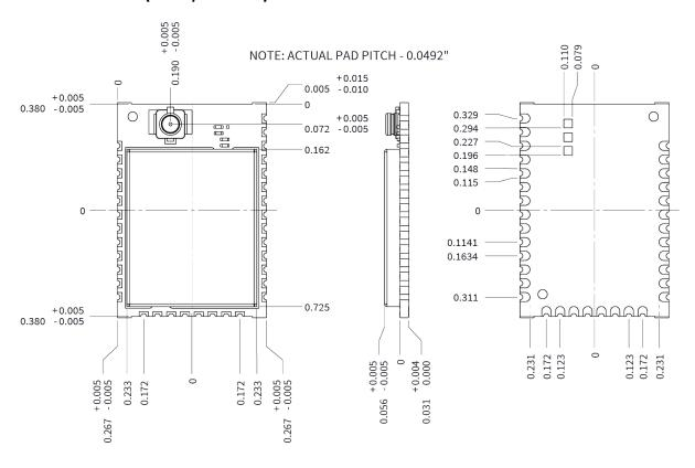
Mechanical drawings XBee 3 micro antennas
