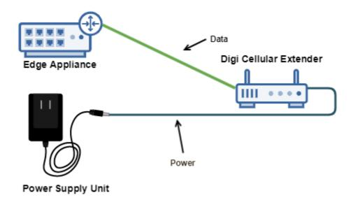
If optimal signal is readily available within range of a power outlet, Digi's Cellular Extenders can be connected directly to the included power supply and then integrated into the network using a standard Ethernet cable.
