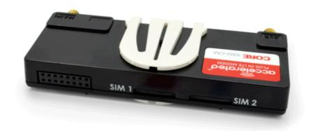
After securing the plug-in module, cover the exposed side of the main appliance using the included faceplate and affix both antennas. The unit is now assembled for cellular network access.
