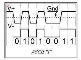
RS-232 is an interface standard, not a data communication standard. It can only go short distances and has very limited driving power. RS-232 was not designed to connect an industrial controller to a computer 100 feet away in another room.
