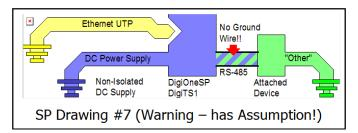
Using a shared DC power supply instead of the AC/DC supply from Digi means the Digi One SP device's RS-422/485 circuit is now referenced to the power-supply ground. While you still have the potential for damaging ground-loop currents, the RS-422/485 chips have thousands of OHMs of impedance. This reduces the likelihood of damage.
