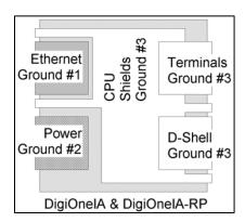
The Digi One IA device includes specific DC-to-DC isolation. The devices accept a 10 to 30 VDC supply and internally isolate that DC power by at least 500 V. Add to this the inherent isolation of IEEE mandated UTP Ethernet and the Digi One IA line is a product with three distinct grounds. If you use the 802.3af powered Ethernet option, this is also isolated internally so it remains related to the Ethernet Ground #1 above.
