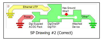
The Digi One SP device is used with an isolated AC/DC supply that creates a RS-422/485 circuit with floating ground. The ideal wiring includes an explicit ground wire to tie the Digi One SP device to the other ground. So your RS-485 two-wire becomes three, and four-wire becomes five. Discussion of the three grounds shown is the same as for SP Drawing #1.
