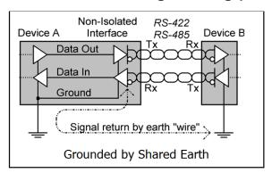
In an office environment, most RS-422/485 devices work with the notion of a grounded power supply. This is because, within a residential or commercial environment, all devices must reference themselves to the one common "safety earth" or "physical earth" (PE). The effect is
