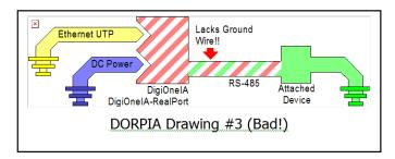
Will the Digi One IA device still work without this connection? Most likely, yes. However, its long-term reliability and survivability will be reduced. The problem is you have added a fourth ground—that of the floating Digi One IA device—and are improperly linking it by RS-485 to the remote RS-485 device. You have not followed TIA/EIA-485A requirements and included a signal return.
