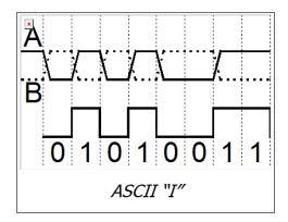
RS-485 is a half-duplex data communication standard that can be used for point-to-point or multi-drop applications. It uses twisted wire pairs. Data is transmitted by a differential voltage signal. The two wires in a pair are not a loop. Both are '+' (positive) signals sourcing current to a
