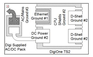
Digi multi-port devices do not include internal DC-to-DC isolation. As far as grounding, isolation, and surge protection goes, they are nearly identical to the Digi One SP device (for more information please read section 5). The one big difference is that 2 to 16 serial ports all share a common ground with the DC power supply.
