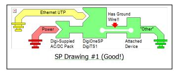
The Digi One SP device used with an isolated AC/DC supply allows the floating RS-232 circuit to readily link and reference itself to the remote device's notion of ground. Given the sensitivity of RS-232 to ground loops, using an isolated DC supply with the Digi One SP device is always the preferred solution. Digi One SP Drawing #1 clearly shows this situation. Three distinct grounding systems are created. How these systems are linked externally is not our concern—our design works regardless.
