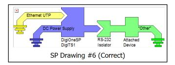
The ideal design when using a non-isolated DC power supply with the Digi One SP device is to add an external RS-232 isolator. These break the ground path and prevent ground loop currents through the RS-232 cable. Cost for external isolators ranges, depending in part on what features they include. For example, some include LED indicators, special connector types, and/or serious surge protection.
