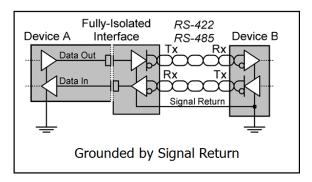
When either device in the RS-422/485 link has an isolated ground, then "a third conductor connecting the common leads of devices" is required. This is when the "signal ground" pins or terminals of the devices are connected. This drawing shows optical isolation in the RS-422/485 port, but the same concept applies if the power supply is isolated.
