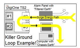
This is really the same problem we discussed with the Digi One IAP device used as a two-port device. But because two, four, eight, or even 16 devices are involved, the probability of killer ground loops occurring is much higher. If the connected devices are all the same make and model from a single vendor, killer grounds are less likely. However, if you are mixing devices from various vendors, then you should assume killer ground loops are highly probable.
