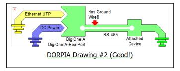
The Digi One IA device's floating RS-422/485 port complicates cabling a bit. By definition, the isolated Digi One IA device does not meet TIA/EIA-485A's Option #2 for signal return by "connections in each, using equipment to an earth reference." So we must meet TIA/EIA-485A's Option #1 for signal return by "a third conductor connecting the common leads of devices." This means we need three wires for RS-485 "two-wire" operation and five wires for RS-422 or RS-485 "four-wire" operation.
