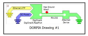
The Digi One IA device's floating RS-232 circuit readily references itself to the remote device's ground. This is ideal for complex or multi-vendor systems. While this Digi One IA RealPort wiring drawing (#1) shows three separate grounds, it doesn't matter how they relate. In most situations they will have identical voltage potentials. But even if fault conditions disturb this, it's not a concern.
