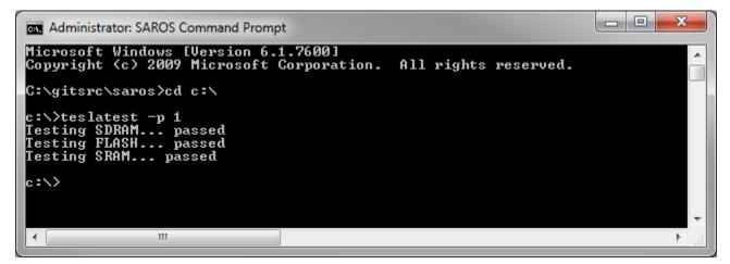
If the SDRAM, FLASH or SRAM test fails then the product should be returned via RMA. When requesting the RMA please include the appropriate fail reason:
