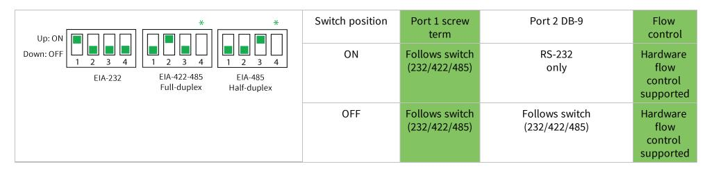
If switch 4 is up, the termination resister is connected. If switch 4 is down, the termination resistor is not connected.
