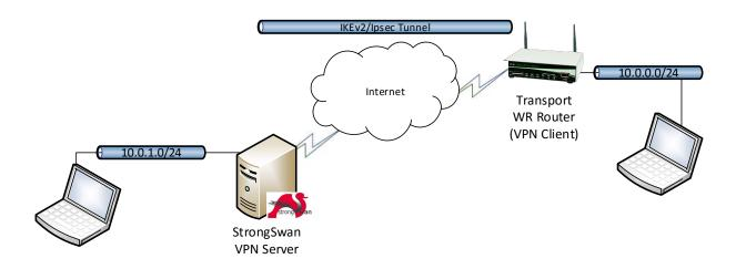
This guide details the steps involved in configuring a Digi TransPort router to act as an IPsec VPN client to a StrongSwan appliance configured as an IPsec VPN server using IKEv2 and Certificates authentication.
