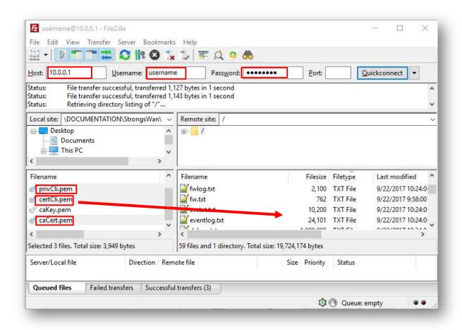
In this example, in order to upload the files, the connection to the Transport is done on the local LAN (so using the ETH o IP address of the router).
