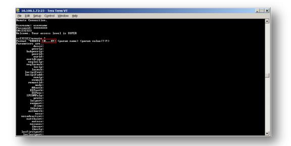
Send the following command: **eroute ?** (if the command result still shows : EROUTE <0...4> (5 tunnels by default) the upgrade was not successful)
