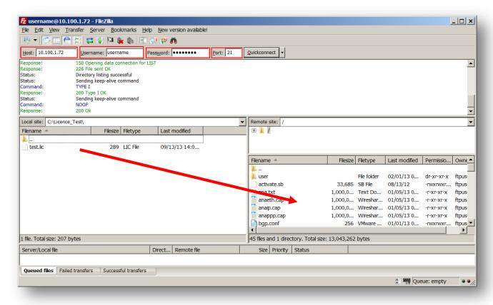
Open an FTP connection to the Transport router that you wish to update. In this example, using FileZilla.
