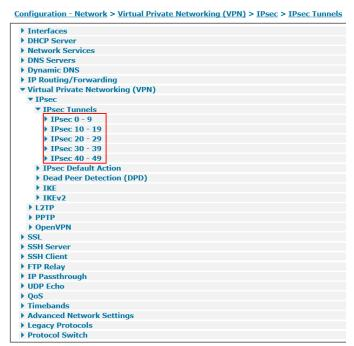
In this example, the TransPort router has been upgraded to 50 IPsec tunnels (PN: **WR-SW-5T50**). The new IPsec tunnels are now available in the web interface.
