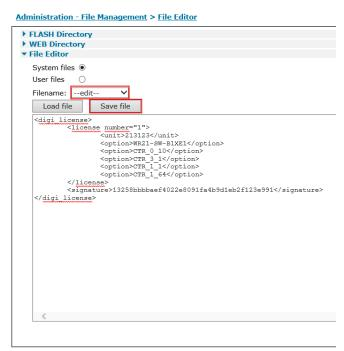
Paste the content of the license file into the file editor box. Double click on the drop down menu, this will allow you to type the file name. Enter for example test.lic
