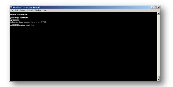
Log in using an account with access level **SUPER** and type **xmodem test.lic** (or the filename of the license file you received) to initiate xmodem file transfer.
