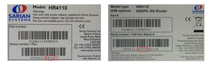
Above are the two label types, the red ellipses highlight where the hardware revisions are located. The table 1 (at the end of this document) details the hardware revision and the corresponding hardware and firmware configuration.
