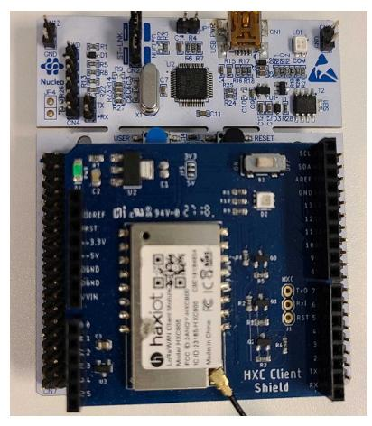
The LoRaWAN Device Developer Kit is configured as a Nucleo Board with an Arduino shield. It contains:
