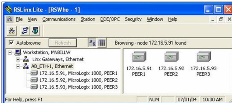
**Note** The Digi One IAP device will show with an “X” as an unrecognizable device if it is not connected, no PLC is attached, or is incorrectly configured (for example, AB Ethernet has not
