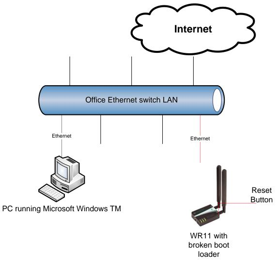
The internet connection is not essential but may be useful during troubleshooting. It is essential that the PC's Ethernet communication interface is configured correctly (e.g. it has an IP address)
