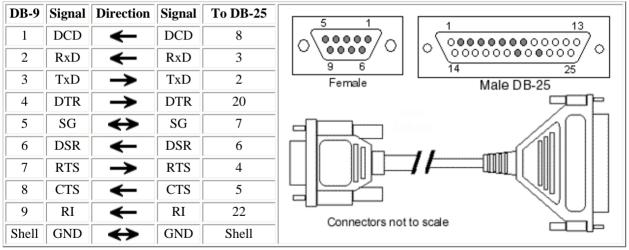
\* Arrows indicate which direction the signal is flowing
