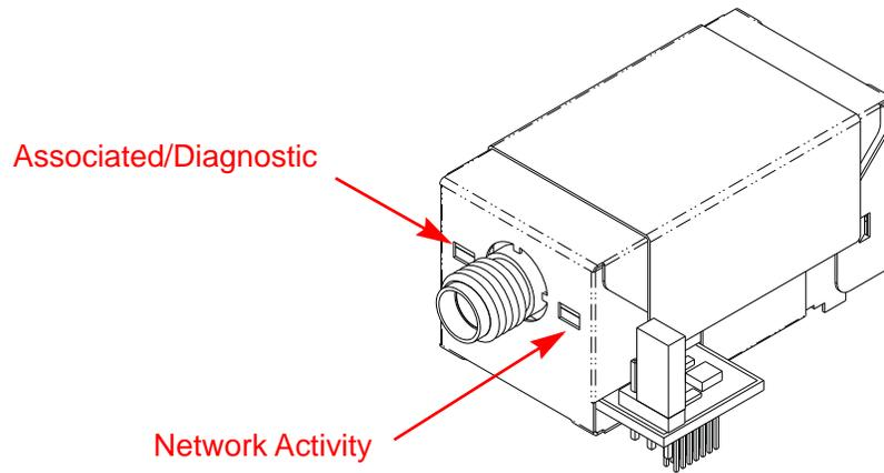
**Note:** The LEDs are the same for a module with or without a JTAG connector.
