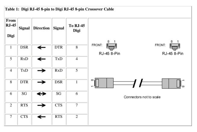
· Arrows indicate which direction the signal is flowing
