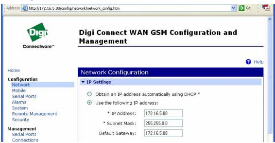
Press **Apply**, and then **reboot** the Digi Cellular Device for changes to take effect. You will lose connectivity to the unit until you reconfigure your workstation to be in the same subnet as the Digi Cellular Device; or use DHCP.
