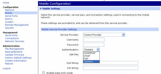
5. If you changed the APN type, reboot the Digi Cellular Device via Administration > Reboot if changes were made to the mobile provider or IP address settings.
