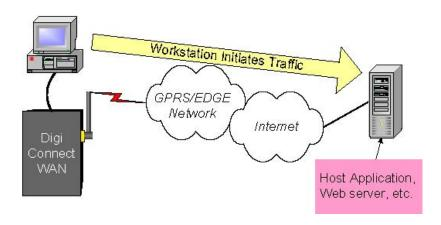
**In-bound Connections** require additional configuration to test. First, not all APN types allow incoming connections. Second, the Digi Cellular Device uses Network Address Translation (NAT)\* to route traffic from the Public IP address on the cellular interface to the Ethernet port's private IP network. NAT provides two main benefits:
