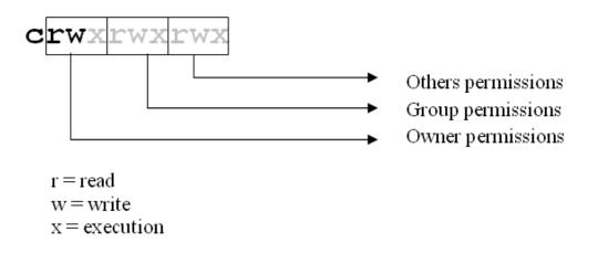
To make the serial port accessible to every user, add read/write permissions for the Group and Others. Open a console and execute the **chmod** command, as **root**, specifying the actual serial port device node in place of /dev/ttyS0.
