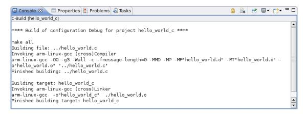
The **Problems** view lists any warnings and errors that occurred during the build process. In such case, the **C/C++ Editor** marks the lines where the problems were detected. The sample application project should build successfully, indicated by the message:
