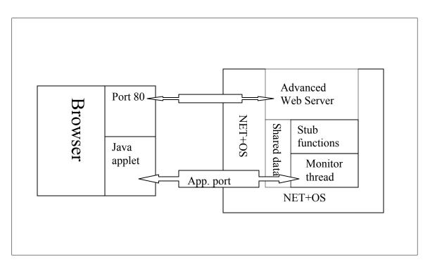
On the left side of the diagram is a browser. This could be MS Internet Explorer, Mozilla firefox or Netscape Navigator. For that matter it could be any browser that supports java applets. The three that I mentioned are the "big three". The block marked port 80 represents standard web pages that would be using the browser for communicating with the advanced web server. I call it port 80 because the standard port for communicating with web servers is port 80.
