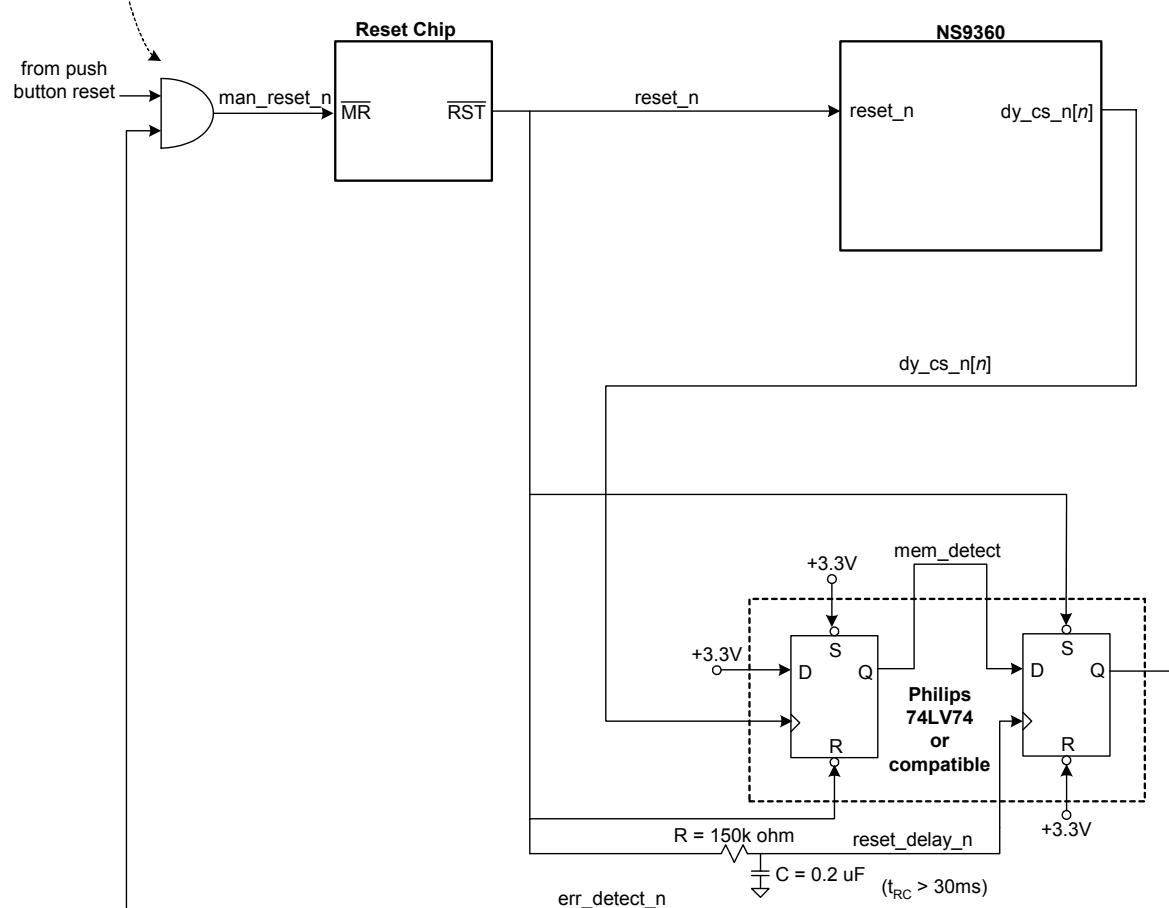
Note: The Philip's 74LV74 has a Schmitt trigger required for the slow rise time of *reset\_delay\_n*.
