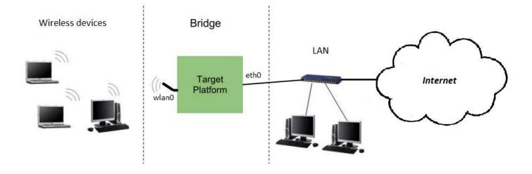
By configuring our platform as a bridge, we will be able to make the three wireless devices connect to the LAN and have access to the Internet.
