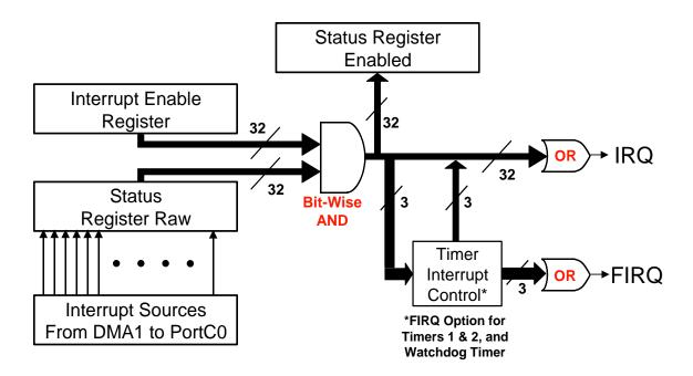
On recognizing the highest-priority interrupt source, the driver temporarily masks out (disables) interrupts from lower-priority sources, ensuring that interrupt service for a high-priority source is not itself interrupted by a request from a lower-priority source. It then re-enables the appropriate exception via the "I" bit in the CPSR to permit higher-priority interrupts to occur and transfers control to the user's interrupt handler (ISR).
