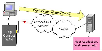
**In-bound Connections** require additional configuration to test. First, not all APN types allow incoming connections. Second, the Digi Connect WAN uses Network Address
