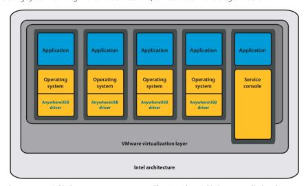
You then connect USB devices to a concentrator. The AnywhereUSB driver installed in the guest operating system manages the connection between the device and the guest.
