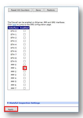
Figure 3.6-4: Firewall settings - Enabling the FW on PPP1
