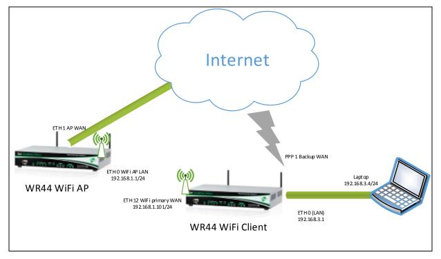
**NOTE**: This AN applies to the configuration of the rightmost TransPort, the Wi-Fi Client. In this this example, the leftmost TransPort represents the AP, which may be an entirely different product.
