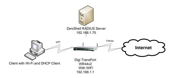
This document describes how to configure a Digi TransPort as a Wi-Fi Hotspot Access Point and Radius authentication to provide Wi-Fi clients with Internet access through Cellular.
