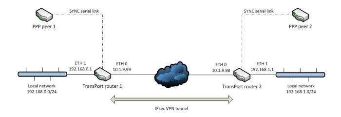
The devices used as PPP peers during the testing of this Application Note were two additional TransPort routers, each with a synchronous serial port. Each PPP peer was connected to TransPort router 1 or 2 via a synchronous crossover serial cable.
