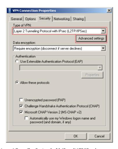
Set Type of VPN to Layer 2 Tunneling Protocol with IPsec (L2TP/IPsec).
