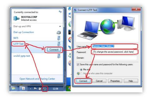
When the PC tries to establish a L2TP tunnel to the VPN Server an IPsec Security Association is established first. This allows the L2TP packets to be encrypted with in the IPsec Tunnel.
