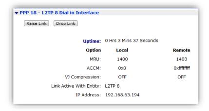
The PC client will now have an L2TP tunnel running PPP on to the VPN Server.
