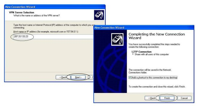
Now some additional settings have to be changed to allow the VPN connection to use IPsec to reach the TransPort. Click on **Properties** and then the **Security** tab, now select **IPsec settings**, tick the 'Use pre-shared key for authentication' option and add in the *Pre\_shared\_key* defined in 2.6.2, now the click **OK** once again.
