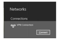
Right-click on the **VPN Connection** and chose **View Connection Properties**. Select the **Security** tab, set the Type of VPN to **L2TP IPsec VPN**, and then click the **Advanced Settings** button.
