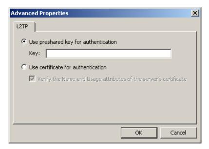
Select **Use preshared key for authentication** and input the shared key in the **Key** field. The Preshared key is the password of the "\*" user that was setup earlier on the TransPort.
