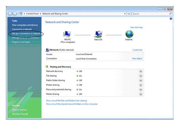
Within it Select **Set up a connection or network.** This will bring up the **Set Up a Connection or Network** wizard:
