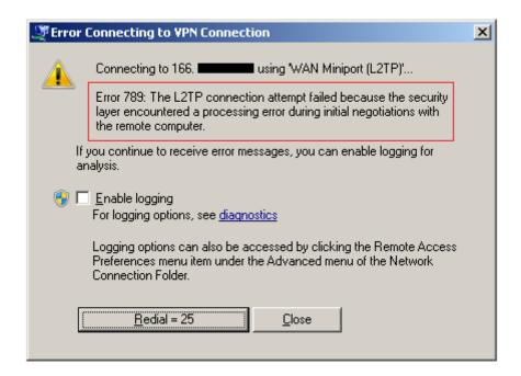
Possible cause #1: L2TP traffic may be blocked somewhere between the PC and the TransPort. Ensure that L2TP is not being filtered out.
