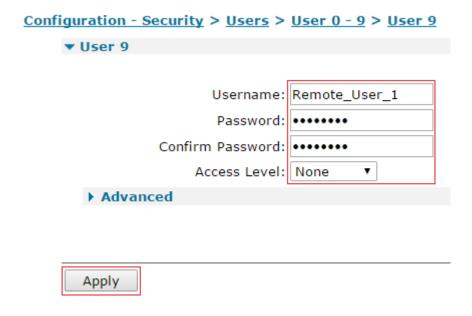
You can assign remote users for general access for the L2TP tunnels to users 3 through 9.
