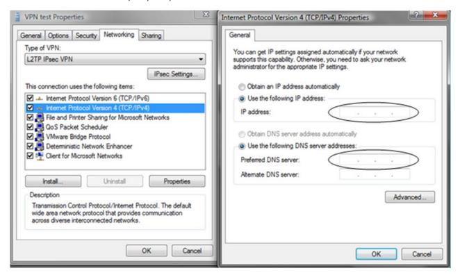
Configure the **IP address** and **DNS server** that the TransPort will use for this L2TP connection. In this example, the IP address configured would be **192.168.63.10** and the DNS sever would be **192.168.63.194.** These values are taken from the configuration in Section 2.6.4, but have been specified manually in the Windows client.
