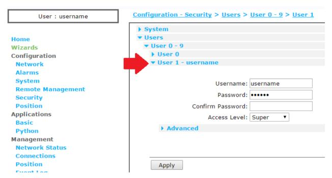
Change the username and password to something more secure than the defaults. If "Super" user access is not necessary, this can also be lowered. More information on the user levels that are supported on the TransPort can be found in the "User Security Settings" section in the <a href="Digi TransPort">Digi TransPort</a> Users Guide on the Digi Support website.
