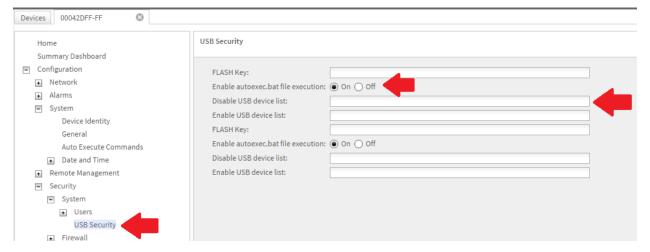
The first field, **Enable autoexec.bat file execution**, enables/disables the use of 'autoexec.bat' files from Mass Storage Devices.
