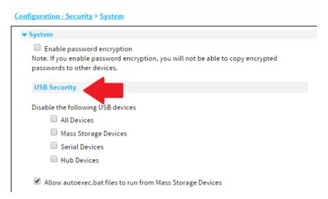
Under this section, there is the ability to turn off the use of all USB devices on the port, or the 3 individual items previously mentioned. If the USB port will not be used, the selection 'All Devices' can be used to disable the use of any USB devices on the TransPort.
