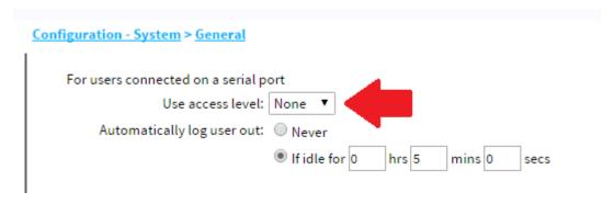
**NOTE**: With the access level of '**None**' chosen, the command '**login**' can still be issued on the serial port to be able to log into the system with the appropriate system user, and the '**logout**' command is used to close the session when finished.
