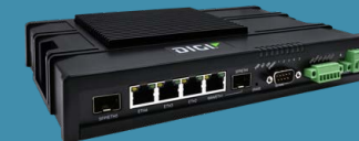
Digi IX40 Cellular Router 5G edge computing industrial IoT router solution, C1D2 certified and purpose-built for Industry 4.0. Offers real-time processing at the edge for manufacturing and precision automation use cases, including advanced robotics, asset monitoring and predictive maintenance.
