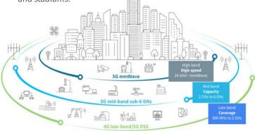
Each band plays a role in delivering the promise of 5G for transforming transit systems. With this three-tiered network architecture, operations teams can prioritize connections based on needs relevant to each use case. Transit systems could reserve high-speed, low-latency communication for mission-critical applications that require real-time functionality while relying on mid-band and low-band tiers for managing the rest of the system's IoT fleet.
