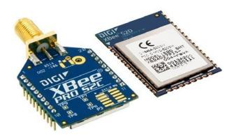
The CAS Tecnologia module, including Digi XBee, helps CAS's utility customers identify incidents of fraud and collect data on energy losses, helping them reduce costs. Today, more than 40,000 CAS products have been produced and delivered to utilities in Brazil.
